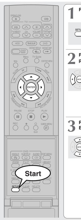
Press SETUP to display the setup menu. When it is already displayed, press O button. (To return to the previous menu) SETUP Press **◄/**▶ to select "Display settings", then press ENTER. Press ▲ / ▼ to select "TV shape", then press ENTER.
